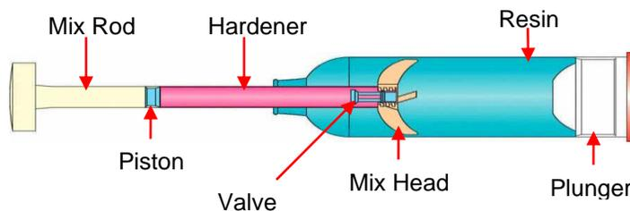
Maximum fluid capacity inside 6" rod = 9cc
