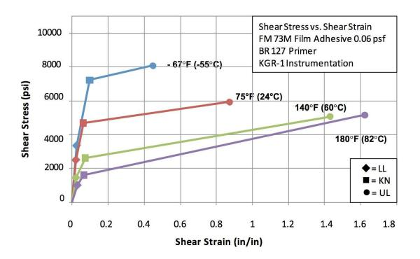
Table 10 | Metal Bonding: Mechanical Properties: KGR-1 Stress Strain Data for FM<sup>®</sup> 73M Film Adhesive, 0.06 psf (300 gsm) with BR 127 Corrosion Inhibiting Primer with Postbond Exposure of 100% R.H. at 140° F (60°C) until Saturated, ASTM D 5656
